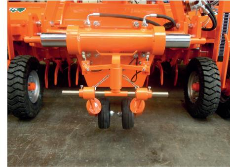
The hydraulic control system ensures that the ridge is built in such a way that the potatoes you plant are located exactly in the middle of it, which reduces the number of green tubers.
