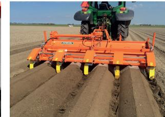
Ensures higher yield by preventing water running towards lower parts of your fields – rainfall stays where it falls. The reservoirs are fully adjustable to your requirements, and are independent of driving speed.
