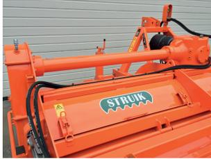
The RF hook-tine rotary cultivator is designed for high power tractors. The drive line is a combination of a gearbox and a chain drive.
