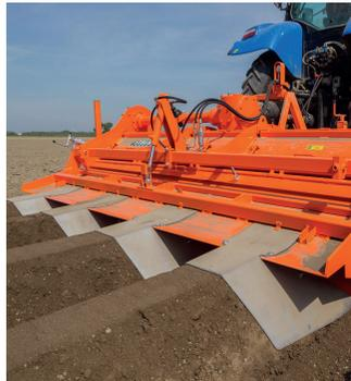
The ridging unit can be equipped with an automatic regulator that maintains constant pressure on the ridging hood, and that produces a lasting ridge with a rigid shape.
