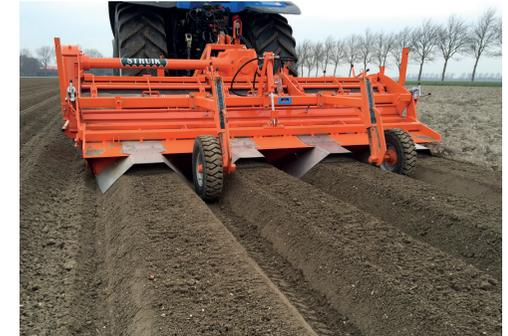
Stainless steel insert plates on the press units for making plateau-ridges, in which you can plant directly.
