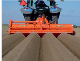
The Striuk ridging system provides voluminous ridges with a capacity of about 620 cm<sup>3</sup>.
