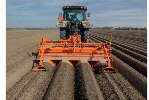
Handle riding tracks easily and quickly with the hydraulic or manual track scrapers.
