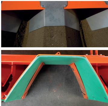
The ridging hood can be equipped with stainless steel press units that allows you to make ridges at a higher speed, and they will keep their shape. With the steel press units coated in Multilene, wear and mud build-up are things of the past. Capacity increases up to 25% are achievable with both systems.
