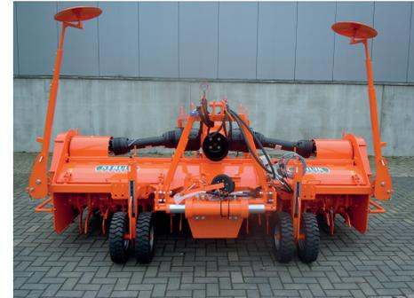
With modifications to the standard frame, the RF is available with a double-sided drive in combination with a maintenance-free centre bearing and a Cat. 3 tensiometer.
